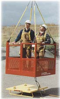
Work platform lifted by a crane using a sling (lifting accessory)
